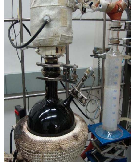
Vacuum distillation unit
