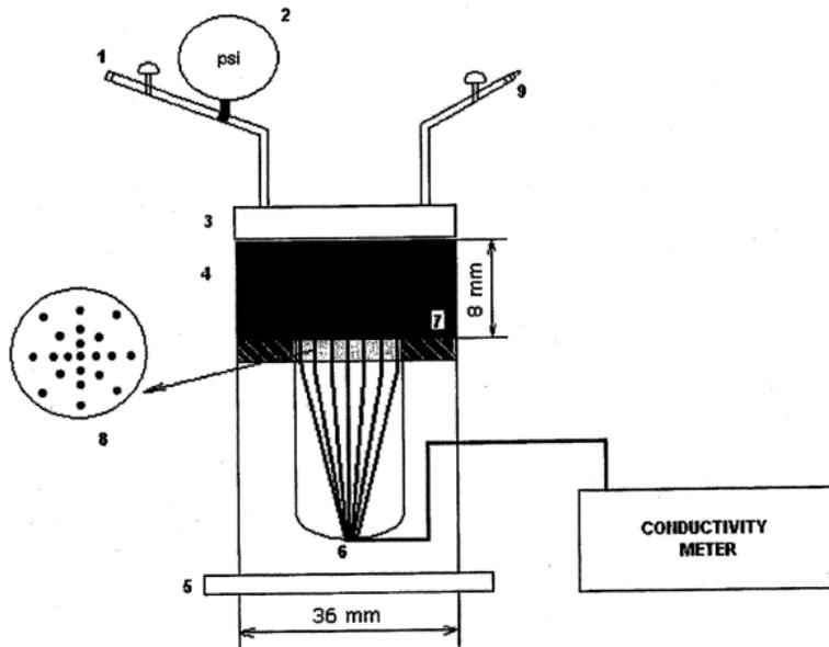
Wettability Test (CWA) using Polarity Switch with readings at 10 second intervals
