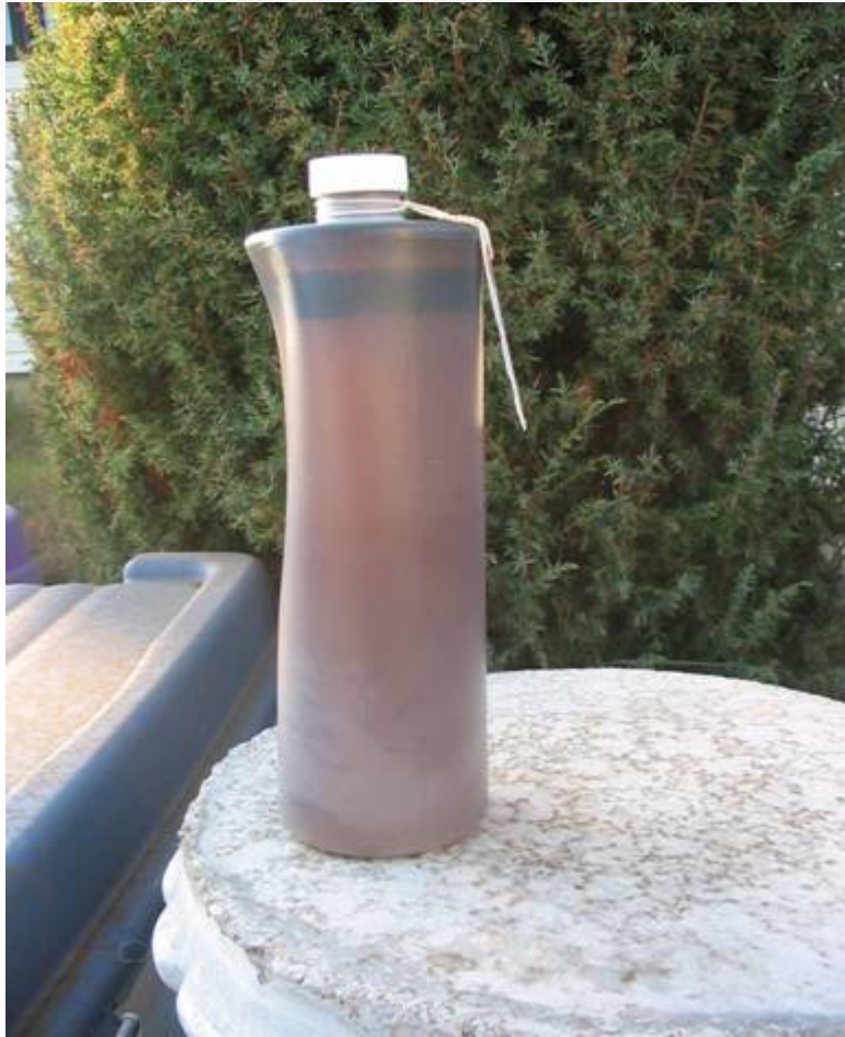
Desalter Effluent Water - Before Pretreatment Program
